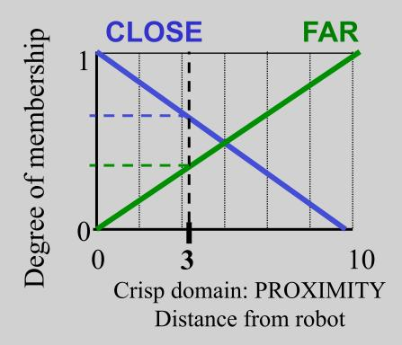
If robot is 3 meters from obstacle, it has a membership in CLOSE of 0.7 and a membership in FAR of 0.3
