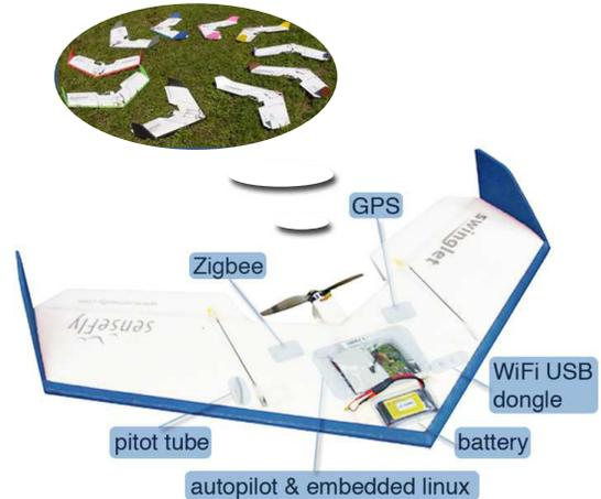
Fig. 3. Aerial swarm composed of 10 flying-wing robots.
