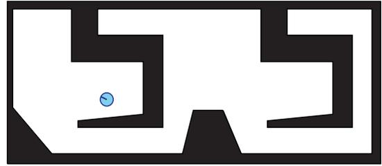
Fig. 1. A robot in a planar environment  $E$ . Its state space is  $X = E \times S^1$ .
