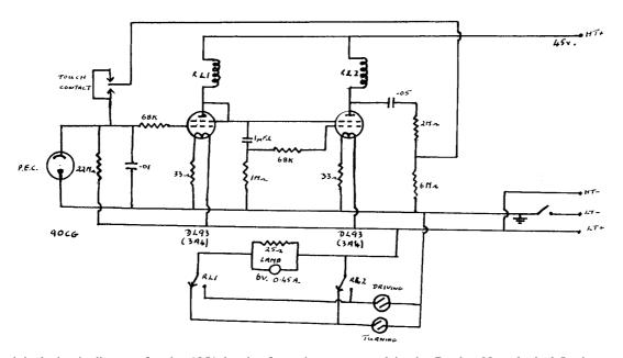
Fig. 3. The original circuit diagram for the 1951 batch of tortoises, preserved in the Burden Neurological Institute archives. It is particularly useful because it gives device types and component values.
