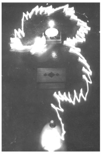
Fig. 7. Elsie demonstrates 'Discernment' by ceasing to respond to the attraction of the candle while dealing with an obstacle.
