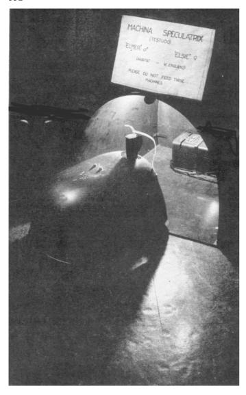
Fig. 1. Dating from 1949, this is probably the earliest surviving image of Elsie, the second tortoise. Through the door of the hutch we can see part of the battery charger. The rather whimsical notice above the hutch reads "Machina speculatrix (Testudo) . . . Habitat – W. England. Please do not feed these machines."
