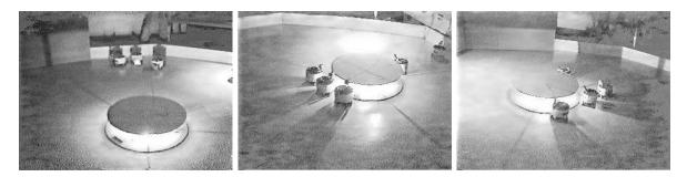
Fig. 8. Shown are five robots pushing a round box from its initial position first towards a goal-light in the right of the picture and then towards a goal-light on the left of the picture. The mpeg video from which this sequence was taken is available at http://www.cs.ualberta.ca/~kube/
