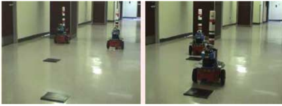
Fig. 4. Physical robot implementation of the transportation task. The initial setup of the two robots is on the left. The result when the two robots reach their goal points (indicated by the squares on the floor) is shown on the right.
