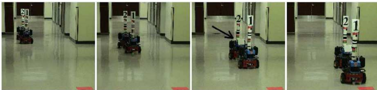
Fig. 8. Partial robot failure. In this experiment, the leader robot R_1 uses its laser to navigate and the follower robot R_2 uses its camera to follow the marker on the leader. During task execution, the camera on R_2 is covered (as indicated by the arrow), and the coalition reconfigures to continue the task. The new solution is that R_1 uses its camera to guide R_2 to the goal. Over ten trials, the average time for these experiments was 112.6 s, with standard deviation of 2.63 s, compared to the no-failure experiment time average of 96.1 s, with standard deviation of 1.45 s.
