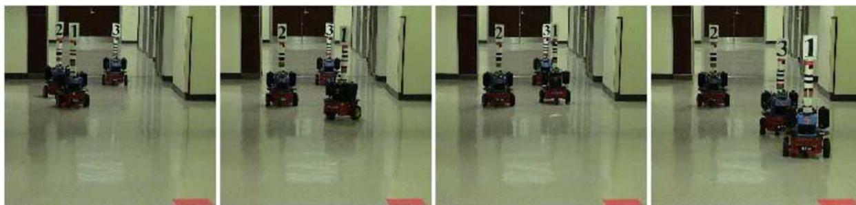
Fig. 9. Simulated robot failure. In this experiment, the leader robot R_1 uses its laser to navigate and the follower robot R_2 uses its camera to follow the marker on the leader. Then, there is a simulated failure of R_2 and the coalition reconfigures the solution. The new solution is that R_1 goes back to pick up another follower R_3 and guide it to the goal. Over ten trials, the average time for these experiments was 187.1 s, with standard deviation of 5.45 s.
