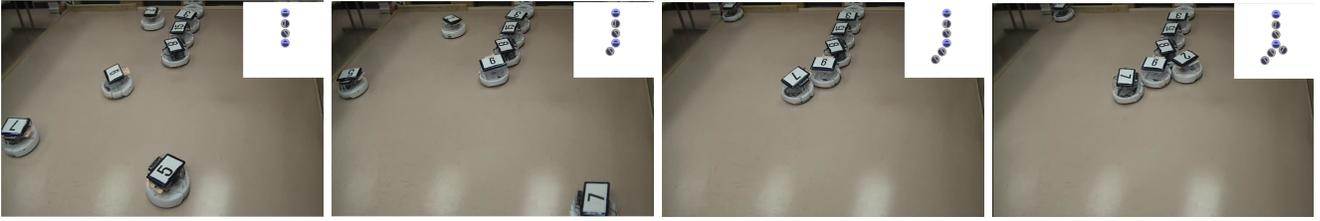
Fig. 3: A typical trial using 7 iRobot Create robots with  $\Delta q = 3$ . The logical tree is shown inset. A branch has been formed in the tree, but edges with robot#2 and robot#7 are not yet complete. Additional robots would need to perform EXTENDEDGE operations for that to occur. This illustrates the asynchronous growth process involved in forming the RRT.
