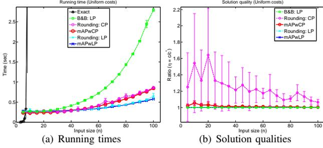
Fig. 4: Running time and solution quality of random instance. (a) The mAPwLP and mAPwCP algorithms are slightly faster than the rounding method whose worst case running time is exponential. (b) The mAPwCP has better solution quality than the rounding method.
