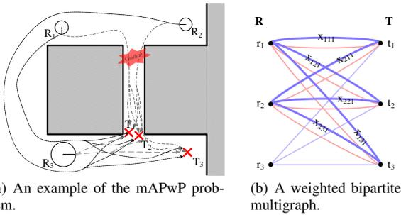
Fig. 1: An example of the mAPwP problem. (a) Robots have multiple ways to reach their destinations. Interference occurs when both  $R_1$  and  $R_2$  use the narrow passage in the center. (b) A weighted bipartite multigraph representation of the example. (Weights are omitted for brevity.) An edge represents a resource (a passage) to perform a task (to reach a destination).
