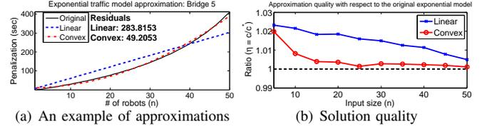
Fig. 5: (a) We approximate a complex exponential function to a linear and a convex quadratic function. (b) Solution qualities when the approximated functions are used for all five bridges.
