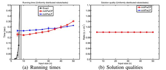
Fig. 7: Running time and solution quality of the multi-vehicle routing problem. (a) The mAPwLP and mAPwCP algorithms quickly produce solutions. (b) The qualities are close to one for both algorithms.
