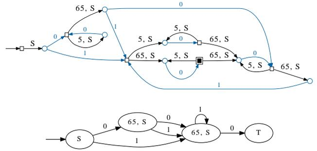
Fig. 6: [top] The I-state graph for the problem of orienting the Fourgon polygon with a binary sensor measuring whether the jaws of the gripper are more than  $x=10.5\text{cm}$  apart or not. Observation arcs are labeled ‘0’ or ‘1’; the latter is returned when the diameter of object in its stable orientation exceeds the distance threshold, and ‘0’ is returned otherwise. (The remainder of the graph follows the format of Fig 5.) [bottom] The most concise plan found.
